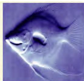
manipulate the relative phases of the X-rays that illuminate and subsequently emerge from an object. They can thus generate phase-contrast images — for example this 50-mm × 50-mm picture of an angel fish — using commercial X-ray sources at much lower intensity and cost, than has previously been possible. The authors note that, as well as improving the detail in X-ray images, their approach could be adapted for use with other low-intensity radiation sources, such as neutrons and ions.
